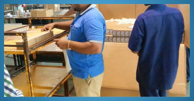
An option is to <u>put the individual items directly on the binning trolley</u> and <u>then label them</u>. A <u>table should be used only to unpack the box</u>. This will save much space and decrease travel time.
