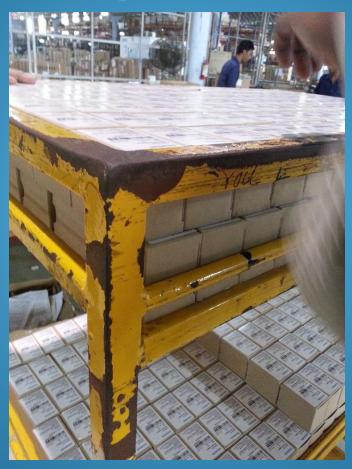
The <u>high railings</u> on the sides of the trolley should be <u>cut off</u> to increase accessibility.
