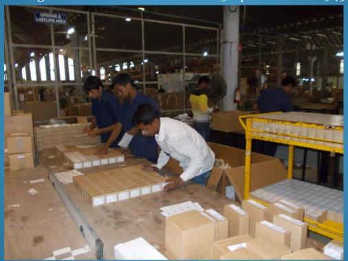
The labeling table should be <u>approximately 37" in height</u>, in order to avoid bending in the neck and back. To account for height differences, the <u>best option</u> would be to install multiple scissor-lift tables on which the unpacking can be performed.
