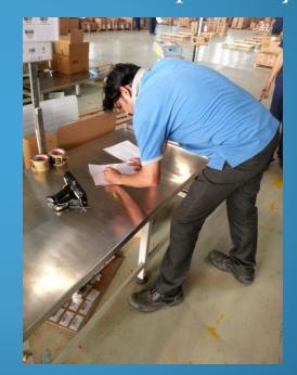
The <u>recommended height for the packing table is waist-height</u> to reduce bending and also allow for comfortable scanner use. <u>A scissor-lift table</u> would be the ideal solution. The use of a <u>handheld or mounted writing pad</u> for placing pick-lists is also highly advised.
