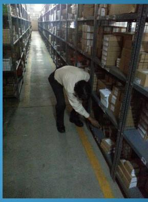
A recommendation is to also consider weight of products while binning. The heaviest material should be placed within the strike zone (shoulders to knees), and lighter material in higher or lower shelves. Portable steps should be available in all aisles, to access material on the highest shelves.
