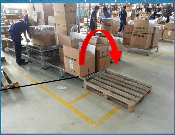
Removing this platform will eliminate the step shown by the red arrow
