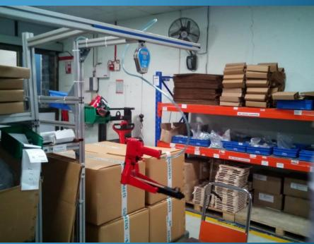
It is highly recommended that <u>overhanging staplers</u> be used (such as in the picture on the right), with <u>spring balancers</u> to ensure efficient and hassle-free operation. Such setups are currently being used at the Siemens location at Kalwa.
