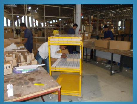
The use of the <u>bottom rack should be eliminated completely</u>. In case of shortage of space, the <u>lightest and fewest number of items should be put</u> <u>on the bottom rack</u>. Also, the picking worker should <u>move around the</u> <u>trolley</u>, rather than bending and stretching uncomfortably to access the <u>racks</u>. <u>Bending should occur at the knees</u>, and not at the back.
