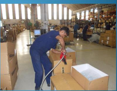
It is recommended that the above activities be performed by keeping the boxes on <u>raised tables</u>. The height of the table should be such that the <u>stapler is held at elbow height</u> (the elbow joint should be at 90 degrees).
